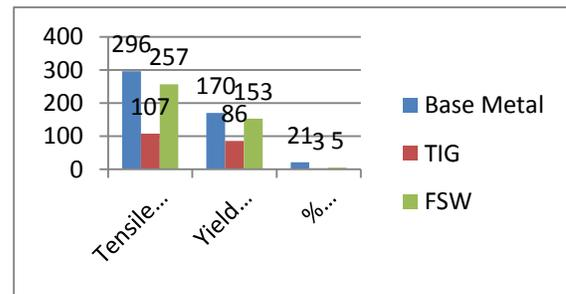
Figure 12: Relationship between base metal, Pulsed TIG welding for sample - 27
