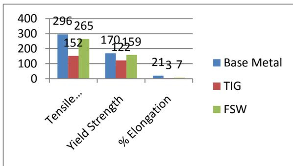
Figure 10: Relationship between base metal, Pulsed TIG welding for sample -3
