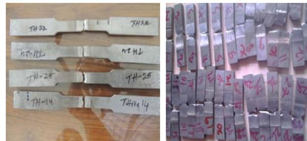
Fig. 7: Tensile and Impact Samples after test
