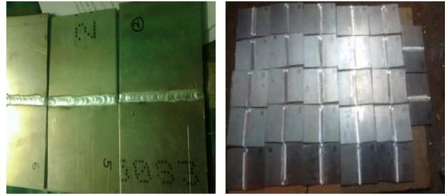
Fig 5: Samples with Weld bead and fsw
