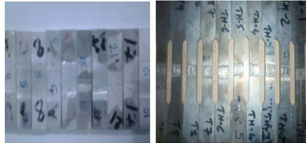
Figure 6: Impact and tensile Test Welded samples cut by EDM
