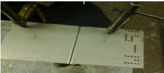
Figure 3: Before welding clapping & Alignment
