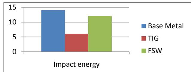
Figure 13: Bar diagram for Pulsed TIG & FSW of Sample 3
