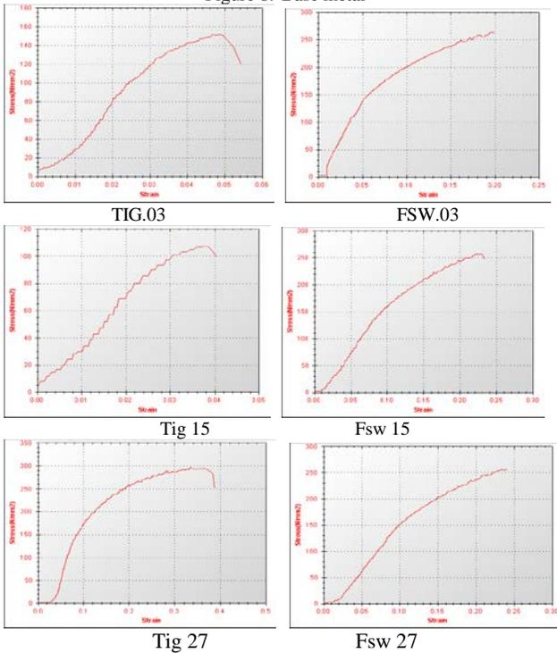
Figure 9: Stress strain curves of FSW and P TIG welding for different samples
