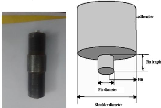
Figure 2: Friction stir welding Tool H13 and Tool geometry
