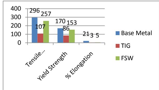
Figure 11: Relationship between base metal, Pulsed TIG welding for sample - 15
