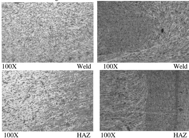
Figure 17: Microstructures for sample Id: 3
