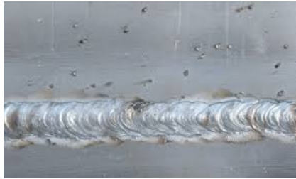
Fig. 1. Welded DSS (double V-groove TIG welded)
