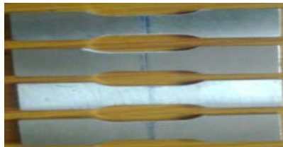
Fig. 3. Prepared Tensile Test Specimen specification
