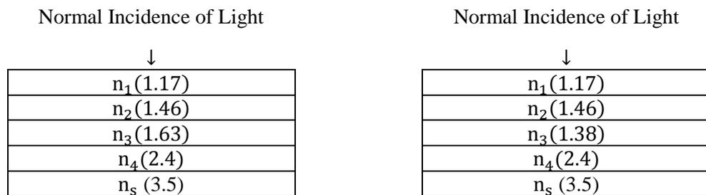
**Figure 5.** Schematic of four layers, optical thickness  $n_1d_1$  and wavelength  $\lambda_0$  for normal incidence of light.
