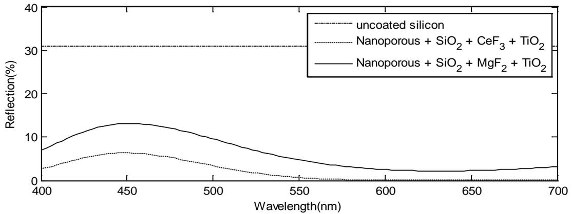
**Figure 6.** Reflectance spectra of four layer antireflection coating on silicon
