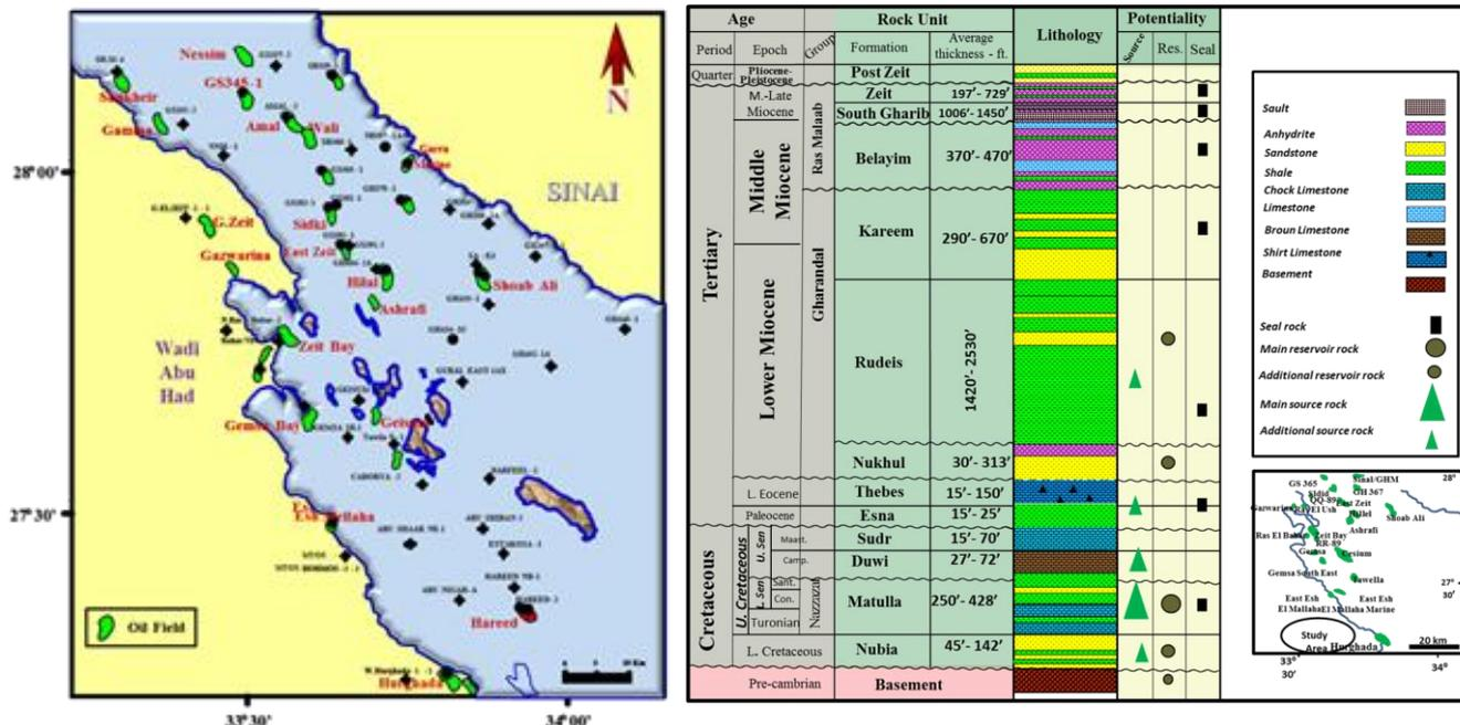
Figure 3: Oil fields distribution of Southern Gulf of Suez district based on well data, and Figure 4: General lithostratigraphic column of West Hurghada district based on well data.
