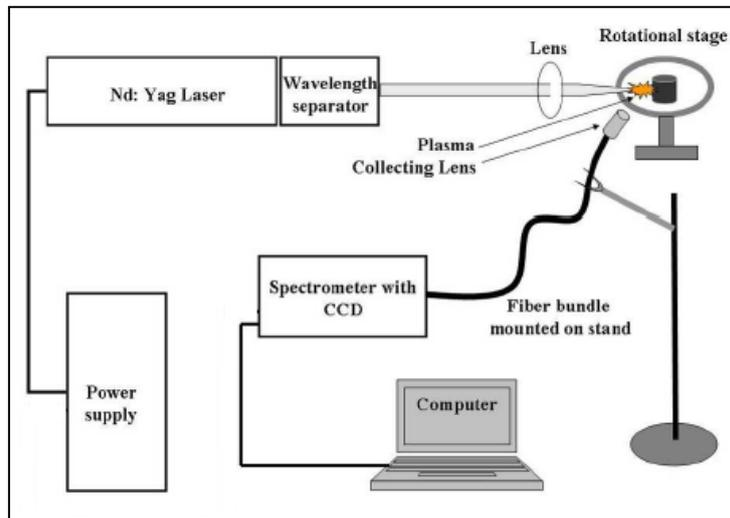
Fig (1 ) The main components of LIPS
