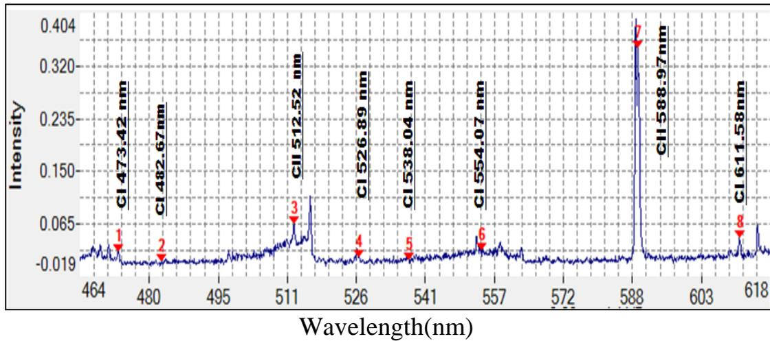
Fig(2 ) The emission spectrum of the produced Carbon (C) graphite plasma in air at normal atmospheric pressure in the region from [464-618] nm for laser energy (334.7 -mJ), and power density ( $6.4 \times 10^6$  MW/  $\text{cm}^2$ )
