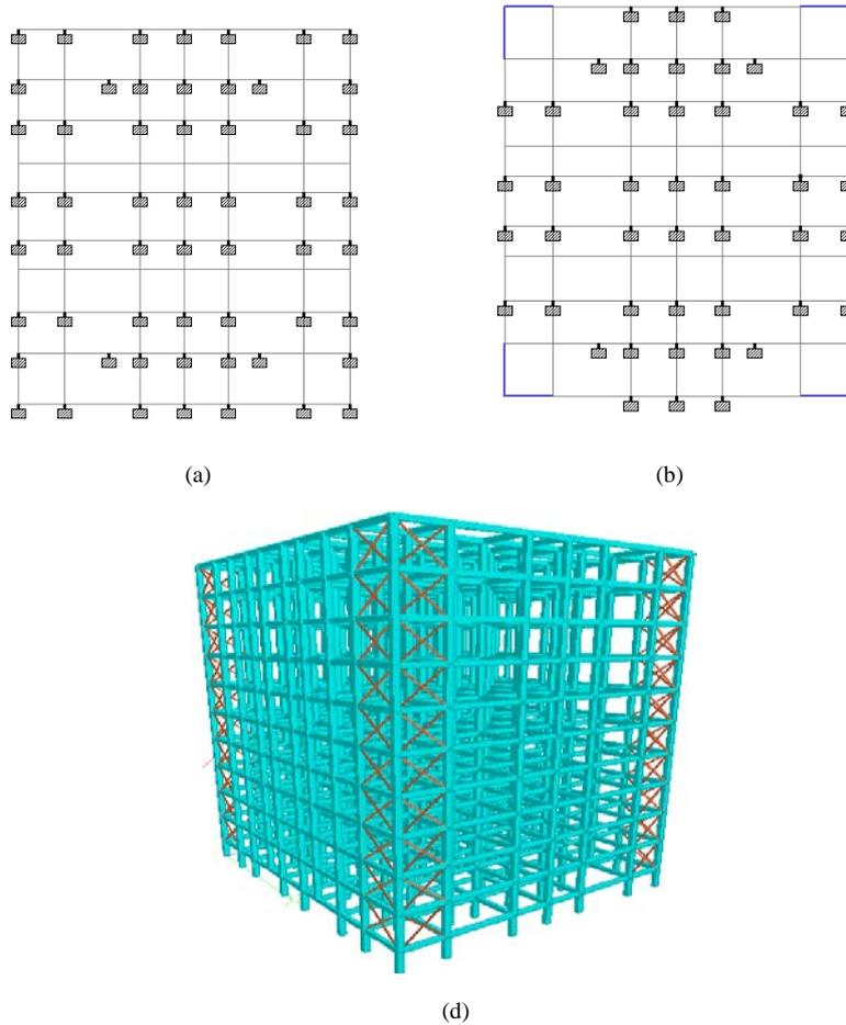
Fig.1 3-D modelling in STAAD.pro software. (a) model-1 without shear wall and bracing, (b) model-2 with shear wall in L-shape, (c) mode-3 with bracing with X type.
