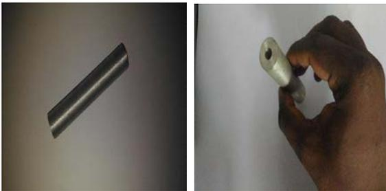
Fig No.3.1 Cast Al-Si cylinder specimen
