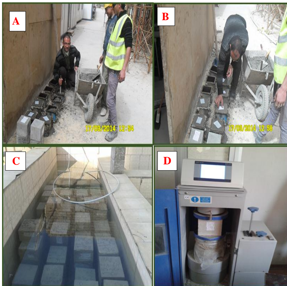
Fig. (8). Stags and methods for preparing concert cubes and testing it according to standards specification.
