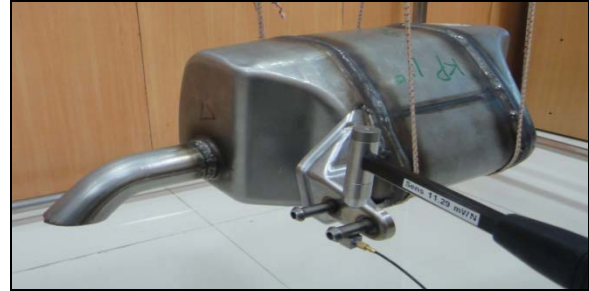
Figure 8. Tri-accelerometer mounted in the hanger 3 for impact testing
