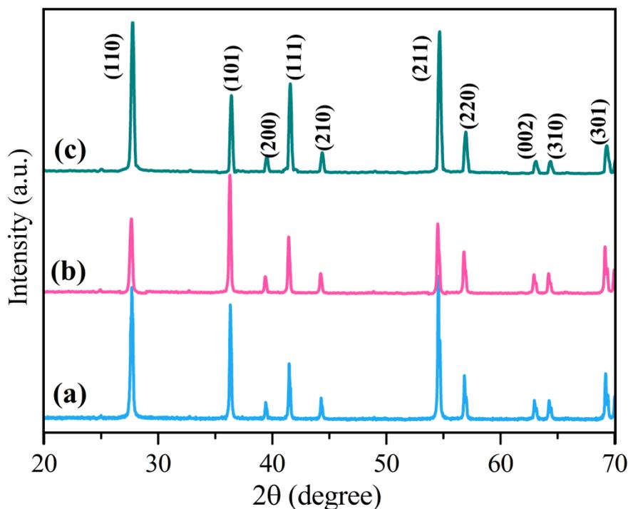
**Fig. 1** XRD pattern of TiO<sub>2</sub> prepared for different hydrothermal treatment time (a) 24 h (b) 48 h and (c) 72 h
