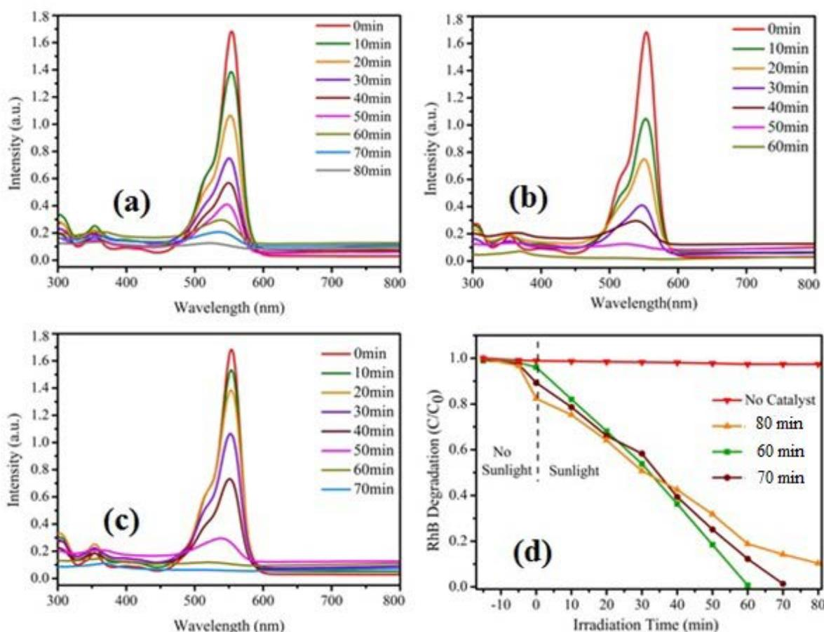
**Fig 5** Photocatalytic degradation of RB solution under sunlight irradiation in the presence of TiO<sub>2</sub> nanoparticles prepared at (a) 24 h; (b) 48 h; (c) 72 h and (d) Comparison of the photocatalytic activities among TiO<sub>2</sub> photocatalyst treated at different HTT.
