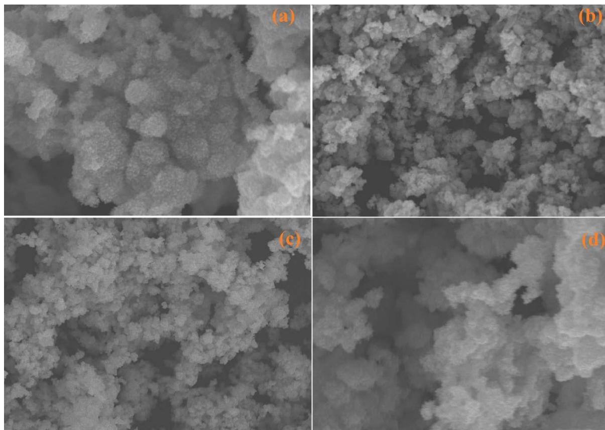
**Fig. 2** FESEM images of TiO<sub>2</sub> prepared for different hydrothermal treatment time (a) 24 h (b,c) 48 h and (d) 72 h.
