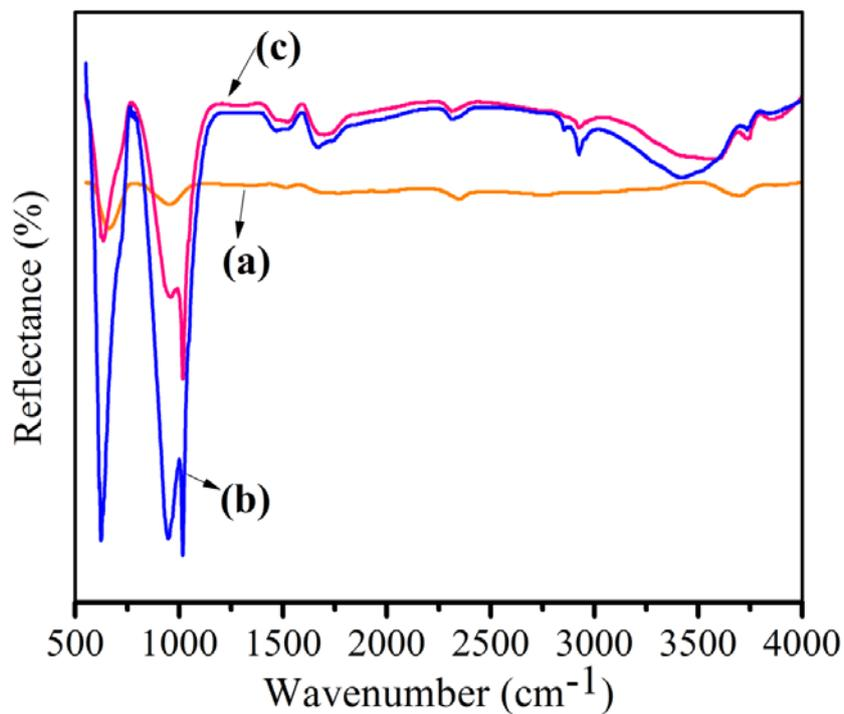
**Fig. 3** FTIR spectra of TiO<sub>2</sub> prepared for different hydrothermal treatment time (a) 24 h (b) 48 h and (c) 72 h.
