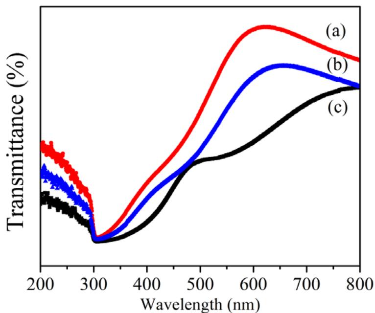
**Fig. 4** UV-Vis spectra of TiO<sub>2</sub> nanoparticles TiO<sub>2</sub> prepared for different hydrothermal treatment time (a) 24 h (b) 48 h and (d) 72 h.
