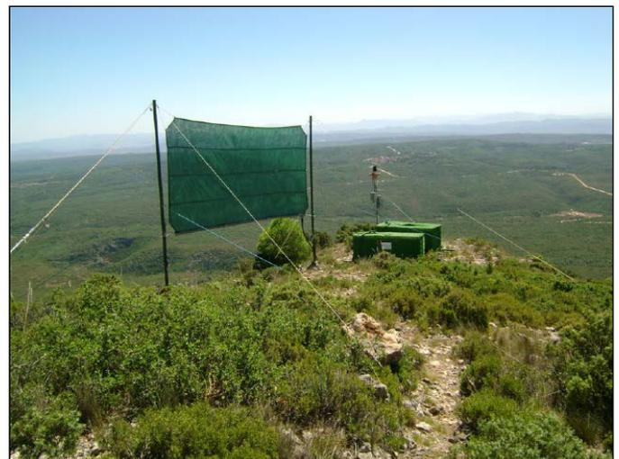
Figure 1. Traditional 18 square meter flat-panel fog collector.
