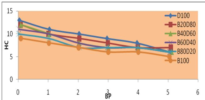
**Fig -6:** Variation of hydrocarbon with brake power
