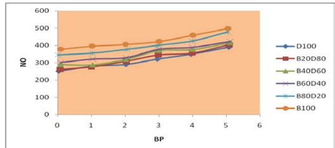
**Fig -8:** Variation of NO<sub>x</sub> with brake power for diesel and corn blends.
