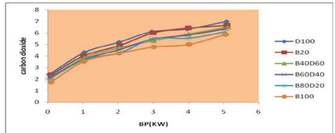
**Fig -7:** Variation of carbon dioxide with brake power
