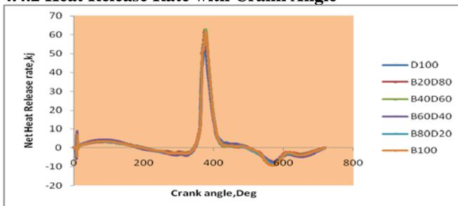
**Fig -10:** Variation of heat release rate with crank angle
