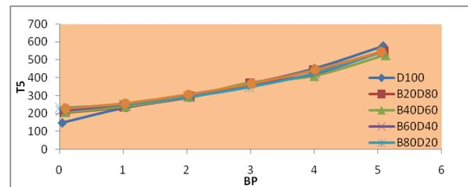
Fig -4: Variation of exhaust gas temperature with brake power
