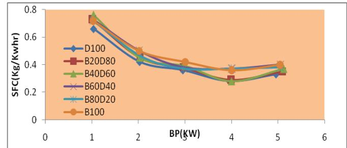
Fig -3: Variation of specific fuel consumption with brake power
