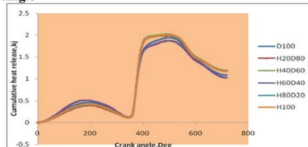
**Fig -11:** Variation of commulative heat release rate with crank angle
