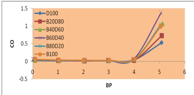
**Fig -5:** Variation of carbon monoxide with brake power
