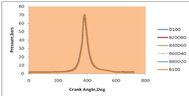
**Fig -9:** Variation of cylinder pressure with crank angle
