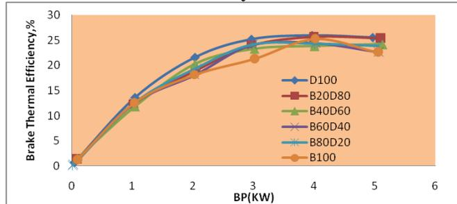
Fig -2: Variation of brake thermal efficiency with brake power
