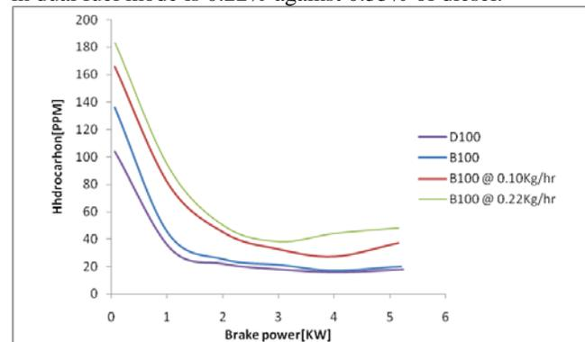
Figure 3.9 variation of unburned hydrocarbon emission with brake power.
