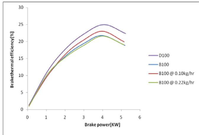
Figure 3.1 variation of brake thermal efficiency with brake power.
