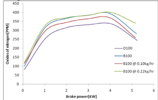
Fig 3.4 variation of oxides of nitrogen emissions with brake power.
