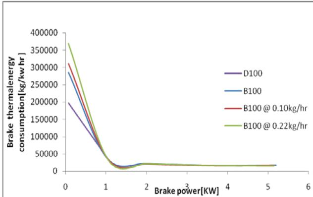
Fig 3.2 variation of brake specific energy consumption with brake power.
