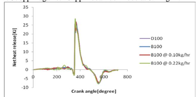
Fig 3.5 variation of net heat release rate with crank angle
