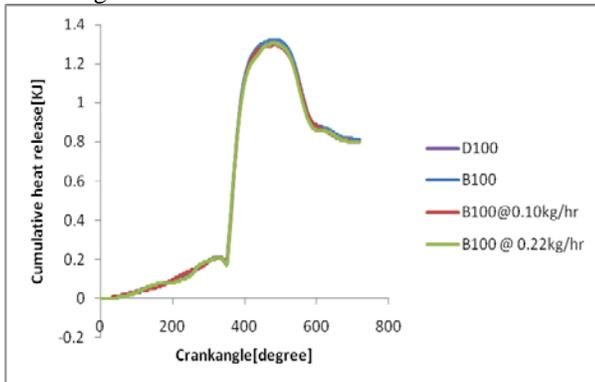
Fig 3.6 variation of cumulative heat release rate with crank angle.
