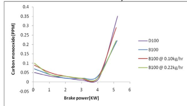
Fig 3.8 variation of CO emission with brake power.
