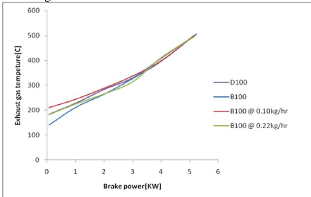
Fig 3.3 variation of exhaust gas temperature with brake power.
