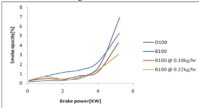
Figure 3.7 variation of smoke opacity with brake power.
