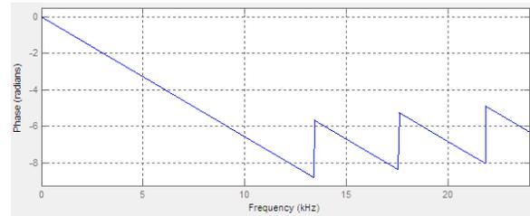
Figure 2: Phase Response of Rectangular Window Technique.
