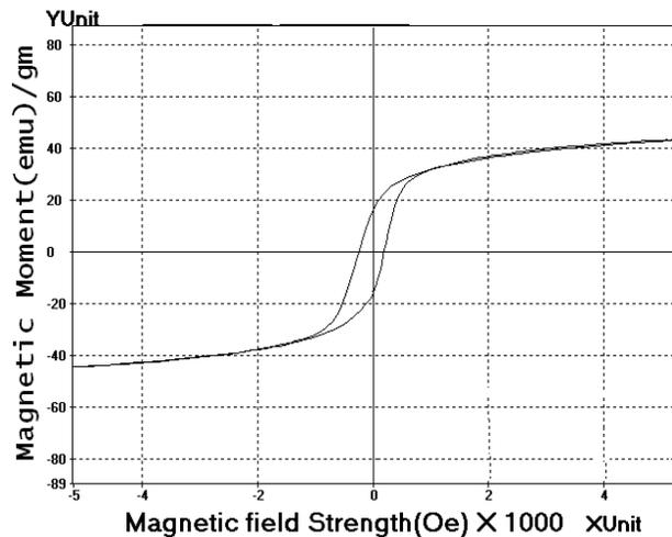
**Fig. 3.** Hysteresis loop for  $Ni_{0.5}Cd_{0.5}Fe_2O_4$  nanoparticles
