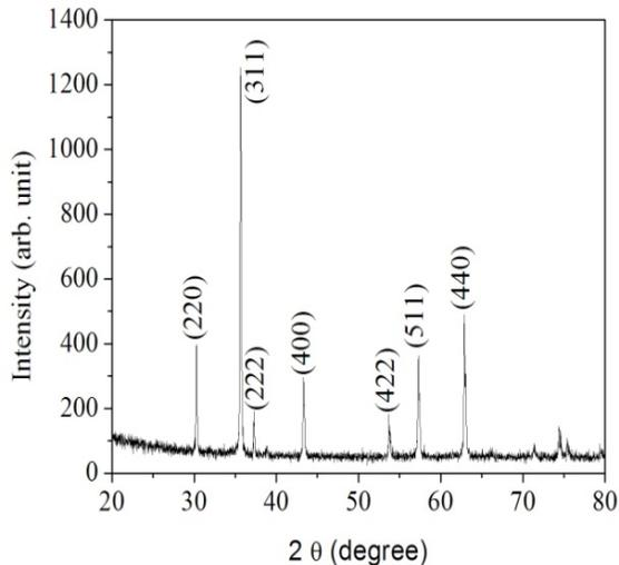
**Fig.1.** X-ray diffraction pattern for  $Ni_{0.5}Cd_{0.5}Fe_2O_4$  nanoparticles
