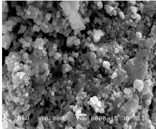
**Fig. 2.** SEM image of  $Ni_{0.5}Cd_{0.5}Fe_2O_4$  nanoparticles
