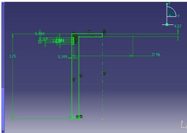
Fig.2.1 Piston Drawing and Dimension
