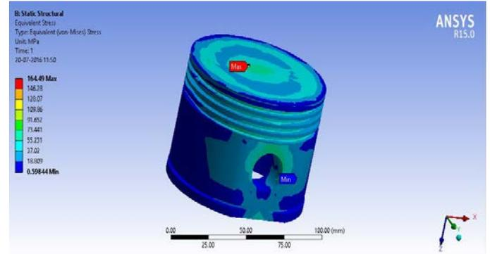
Fig 4.3: static analysis for steel-  $\text{SiO}_2$  material stress
