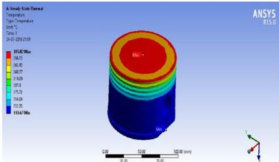
Fig 4.5 : Thermal analysis for steel material temperature distribution
