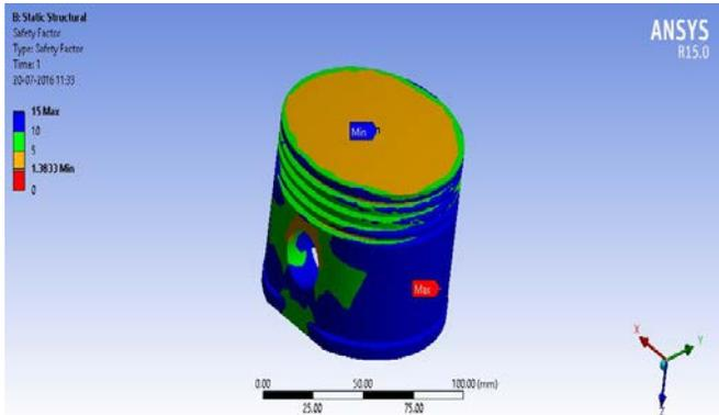
Fig 4.2: static analysis for steel material Factor of Safety
