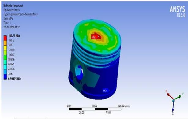
Fig 4.1: static analysis for steel material stress
