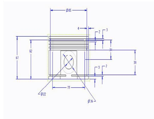
Fig: 3.1 Design Parameters of Piston
