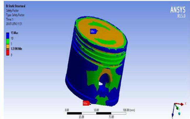
Fig 4.4: static analysis for steel-  $\text{SiO}_2$  material Factor of Safety
