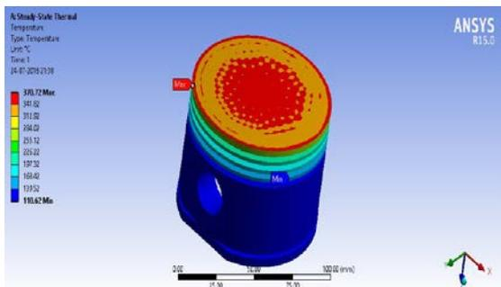
Fig 4.6: Thermal analysis for steel-SiO<sub>2</sub> material temperature distribution
