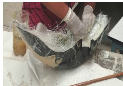
Fig 4.2. Applying layers of fiber on mould
