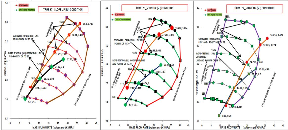
Fig. 5 B60J67, A58N70 and A58N72 Turbo-match- by Simulation & Data-logger – Slope-up Route
