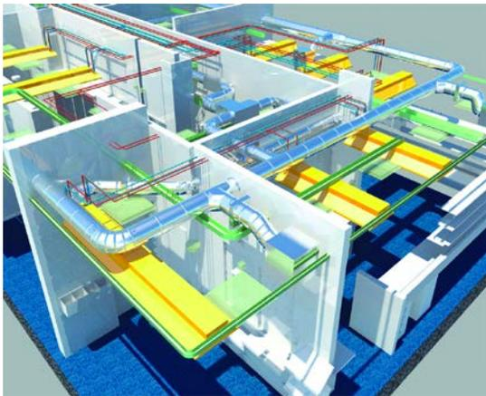
A building information model can contain crucial information about where all the fire-prone insulation is present, where all items which contain chemicals are installed, how is the compartmentalization being done, how is the air ventilated.
