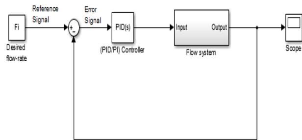
Figure 2: PI/PID controlled flow system
