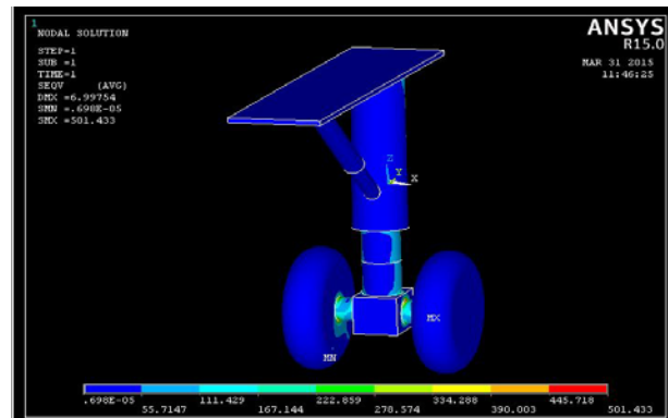
Fig. 8 Titanium 6AL-4V – Stress distribution.
