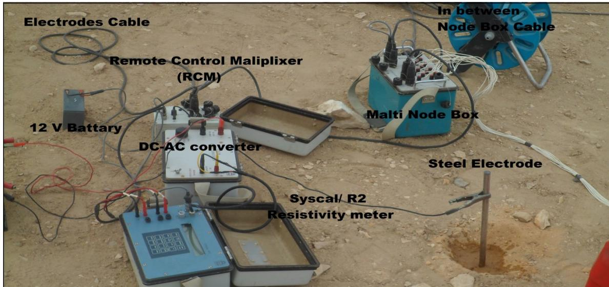
**Figure 3: Instruments used in the geoelectrical surveying and 2-D geoelectrical resistivity imaging**
