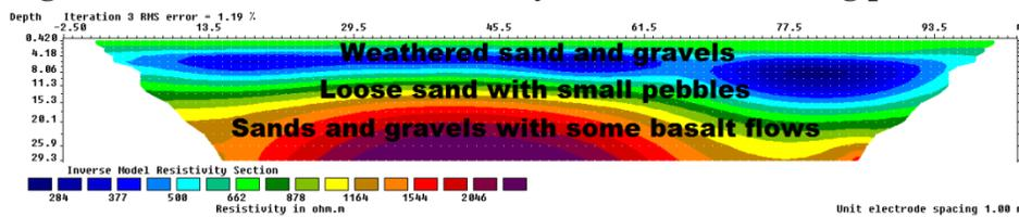
**Fig. (III –8): 2-D electrical resistivity sections No.24 along profiles P4.**
