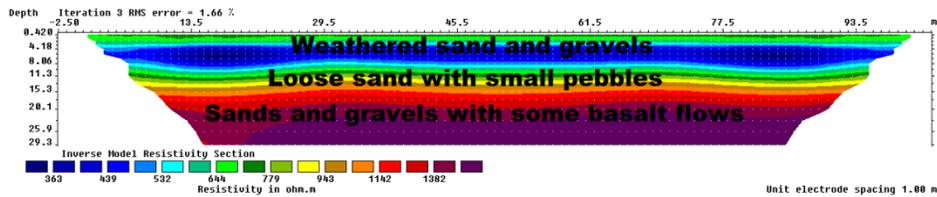
**Fig. (III –6): 2-D electrical resistivity sections No.12 along profile P2.**
