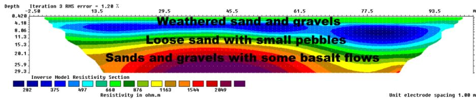
**Fig. (III –5): 2-D electrical resistivity sections No.1 along profile P1.**
