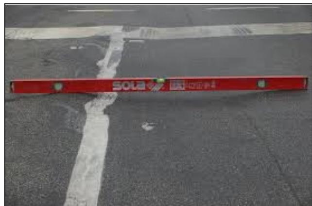
Fig. 1 Measurement of Rutting
