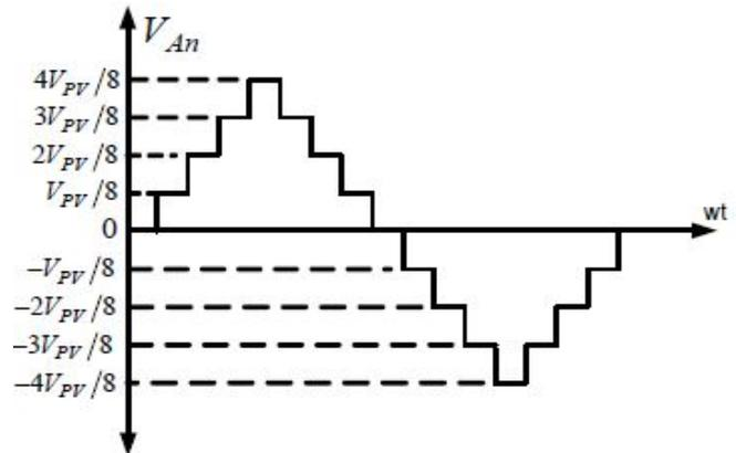
Fig. 3. Proposed topology output voltage waveform
