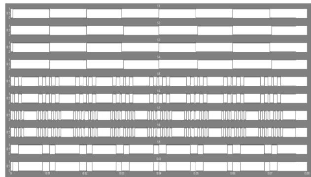
Fig. 7. Switching pattern of switches S1 to S10
