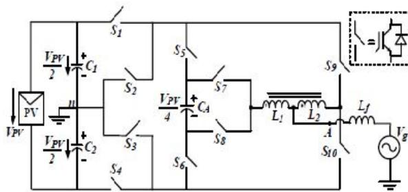
Fig. 2. Proposed hybrid 9-level inverter topology
