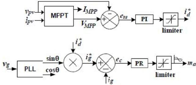
Fig. 5. Control strategy for the proposed 9-level inverter
