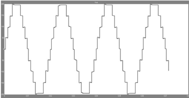
Fig. 8. Output voltage waveform of hybrid 9-level inverter
