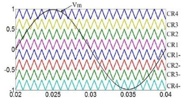
Fig. 4. PWM technique for the proposed 9-level inverter
