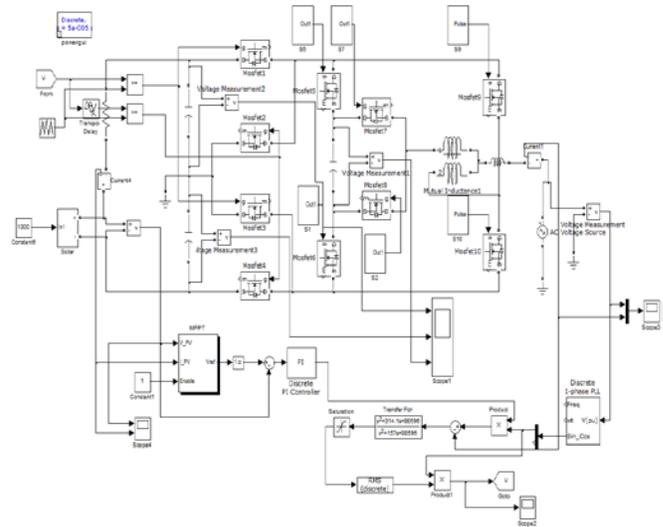
Fig. 6. Simulink model of hybrid 9-level inverter with Grid connected load
