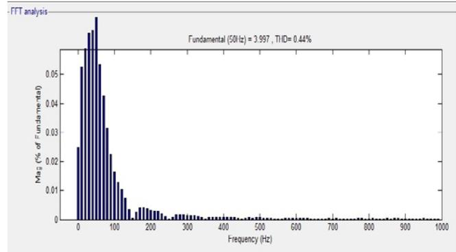
Fig. 12. THD analysis of output current
