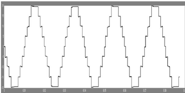
Fig. 9. Output current waveform of hybrid 9-level inverter
