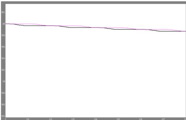
Fig. 10. Input capacitors (C1, C2) voltage waveforms
