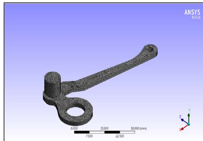
Fig. 2 Mesh model for original shape with 2mm thickness
