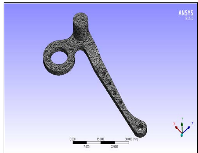
Fig. 3 Mesh model for original shape with 4 holes
