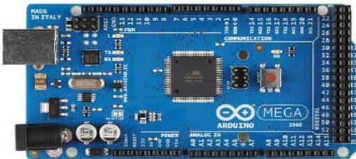
Figure 5. The Arduino Mega 2560.
