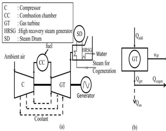
Figure 1.1(a) Schematic diagram of a cogeneration cycle plant (b) Energy flow diagram of cogeneration cycle power plant
