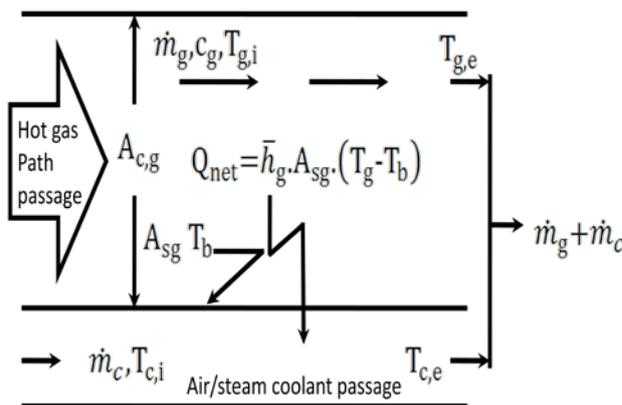
Figure 2.2 Model for open loop internal convection turbine blade cooling
