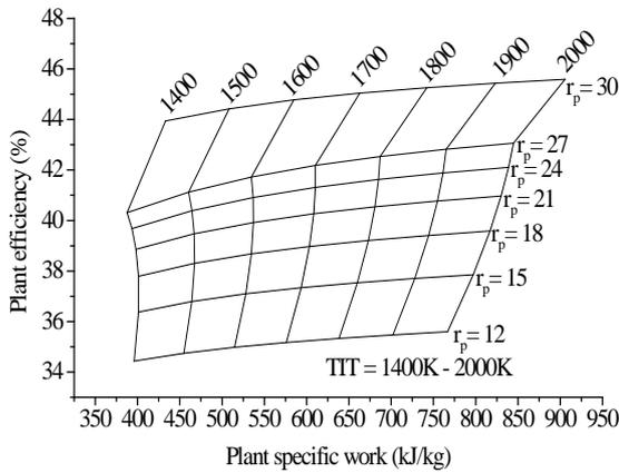
Figure 4.4 Basic gas turbine with open loop steam convection cooling.
