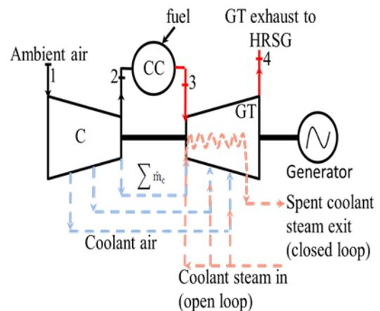
Figure 2.1 Air cooled gas turbine with open & closed loop blade cooling
