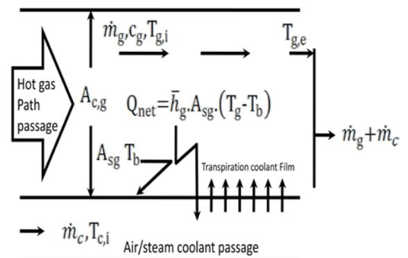
**Figure 2.4 Model for transpiration cooling of turbine blade**
