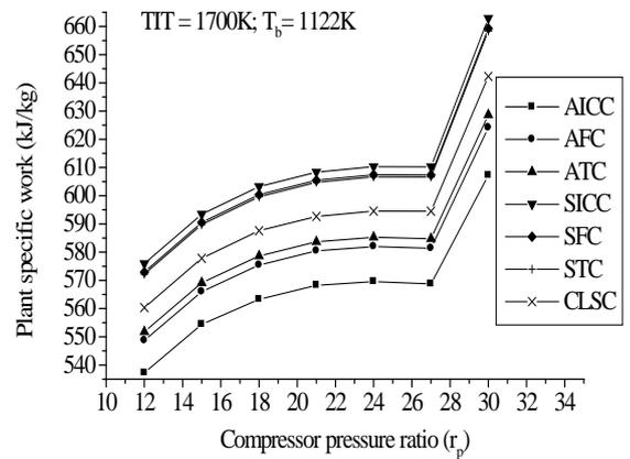
Figure 4.8 Compressor pressure ratio vs. Plant specific work with different cooling means for basic gas turbine.
