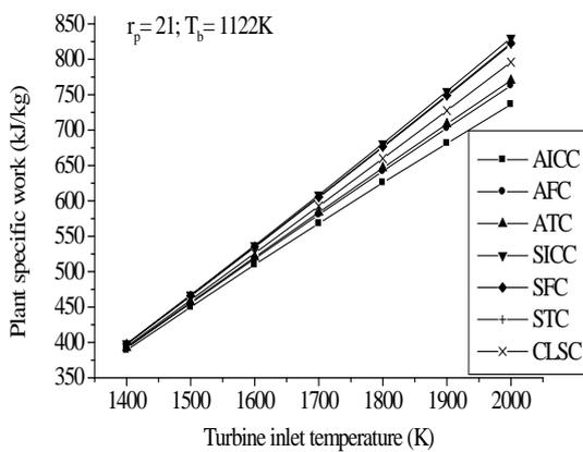
Figure 4.12 TIT vs. plant specific work with different cooling means for basic gas turbine.
