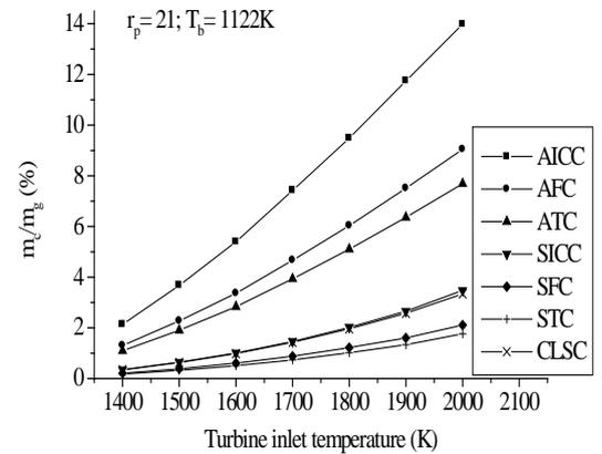
Figure 4.15 TIT vs.  $m_c/m_g$  with different cooling means for basic gas turbine.
