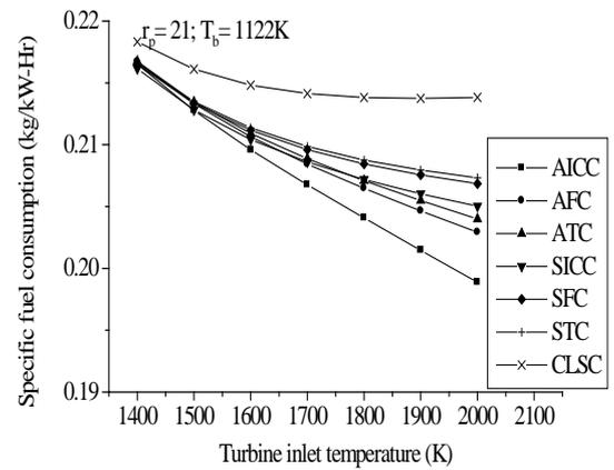
Figure 4.14 TIT vs. SFC with different cooling means for basic gas turbine.
