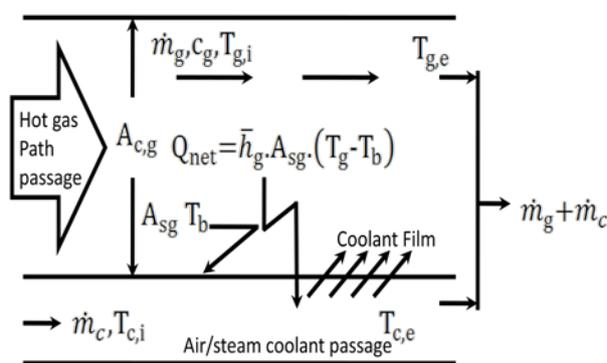
**Figure 2.3 Model of open loop film cooling turbine blade**
