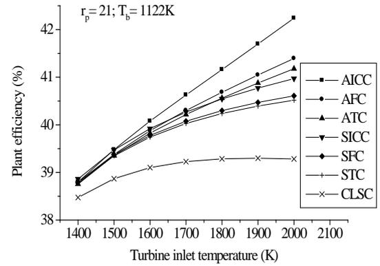
Figure 4.13 TIT vs. plant efficiency with different cooling means for basic gas turbine.
