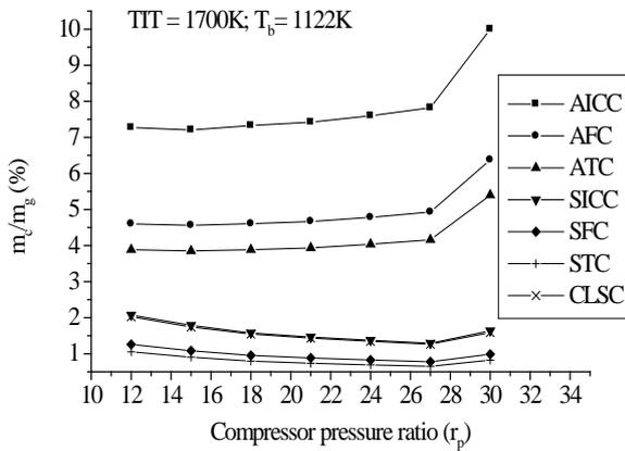
Figure 4.11 Compressor pressure ratio vs  $m_c/m_g$  with different cooling means for basic gas turbine.
