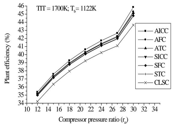
Figure 4.9 Compressor pressure ratios vs. Plant efficiency with different cooling means for basic gas turbine.
