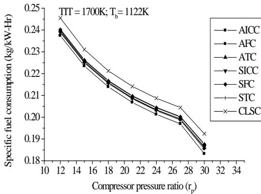
Figure 4.10 Compressor pressure ratio vs. sfc with different cooling means for basic gas turbine.
