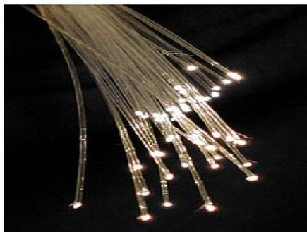
Fig. 3 bundle of optical fibers
