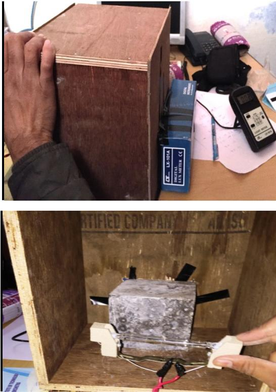
Fig 7 Experimental setup to find light guiding property of light transmitting concrete
