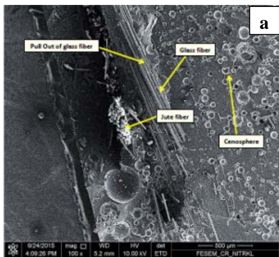
Fig. 10(c) and (d) SEM images of tensile fractured surfaces of 20wt.% cenosphere filled hybrid glass-jute (GJJG) epoxy composites in saline water environment at lower (200x) and higher (1000x) magnification
