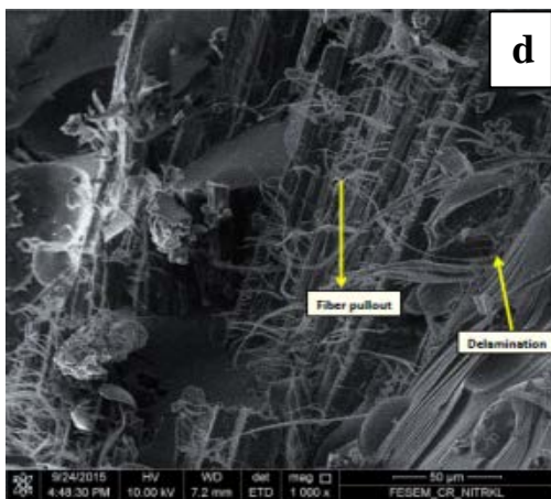
Fig. 10(c) and (d) SEM images of tensile fractured surfaces of 20wt.% cenosphere filled hybrid glass-jute (GJJG) epoxy composites in saline water environment at lower (200x) and higher (1000x) magnification
