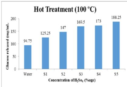
**Fig 3a: Effect of hot acid treatment on sugar release by H<sub>2</sub>SO<sub>4</sub>**
