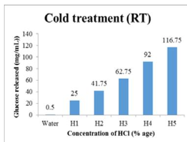
Fig 1b: Effect of cold acid treatment at RT on sugar release by HCl.
