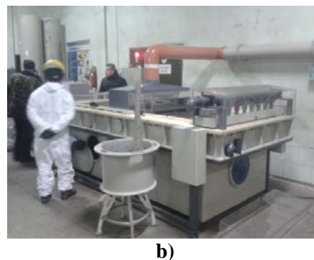
Fig. 2 3D-scheme of electrochemical reactor (a) and the view of the technological testing of electrochemical reactor with 10 kg/h production capacity (b).
