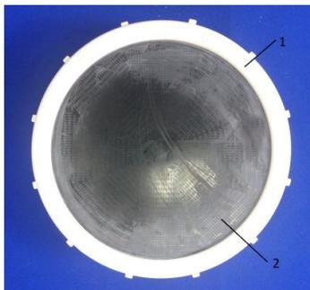
Fig. 3 General view of the porous diffuser
