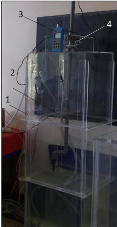
Fig. 10 Water tank with the oxygenometer sensor probe inserted into it
