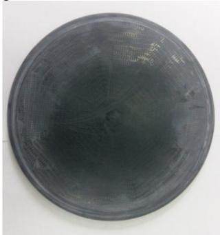
Fig. 2 Elastic membrane of E.P.D.M..
