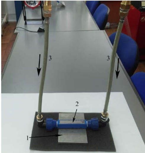
Fig. 3 General view of the fine bubble generator 1 - support plate; 2 - generator body; 3 - compressed air supply pipes.
