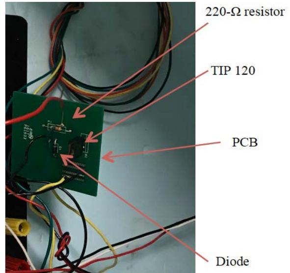
Fig. 4 Printed circuit board circuit.
