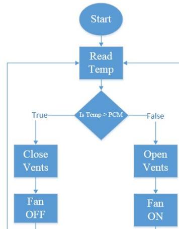
Fig. 5 Flow chart for the microcontroller code.
