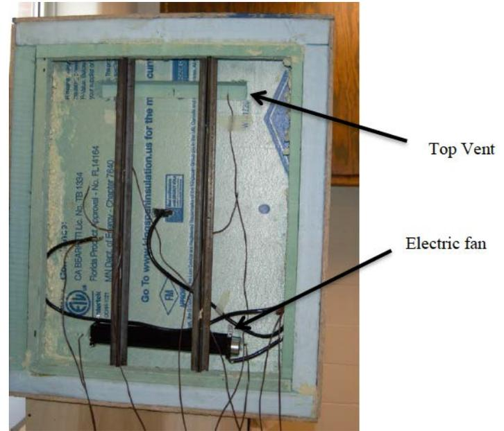
Fig. 7 Picture of the Electric fan in the experimental set-up
