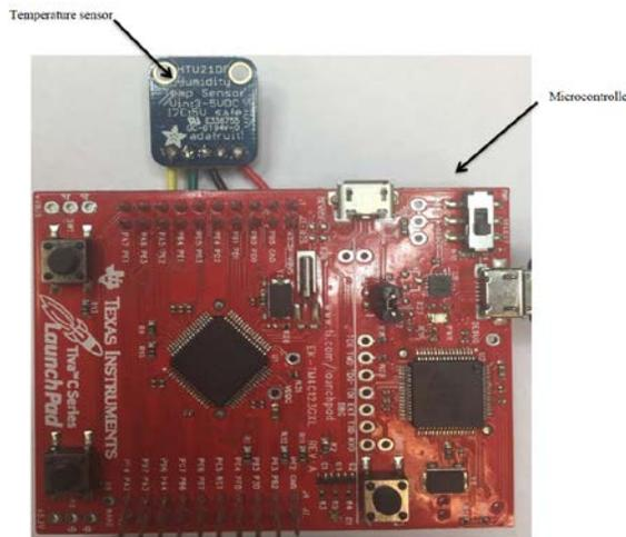
Fig. 3 TM4C123 microcontroller and HTU21D (F) temperature/humidity sensor.
