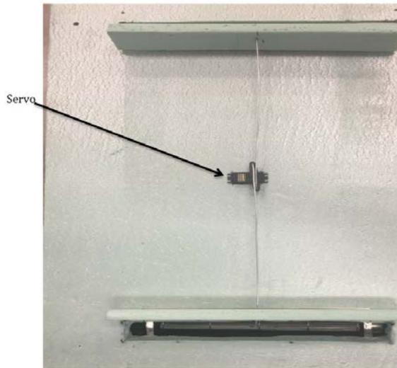
Fig. 6 Picture of the vent system
