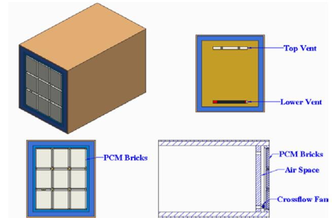
**Figure 2.** 3D Model of Solar Wall
