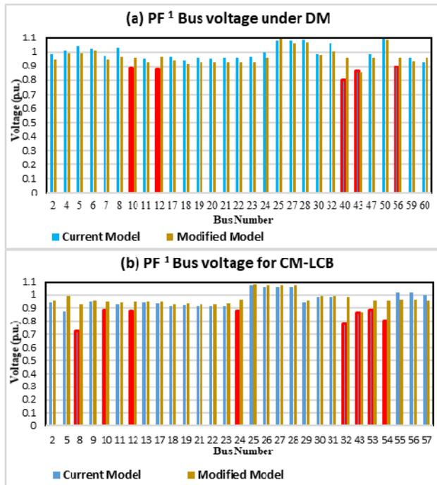
Fig. 12. PF<sup>1</sup> bus voltage comparison between current and modified SIG
