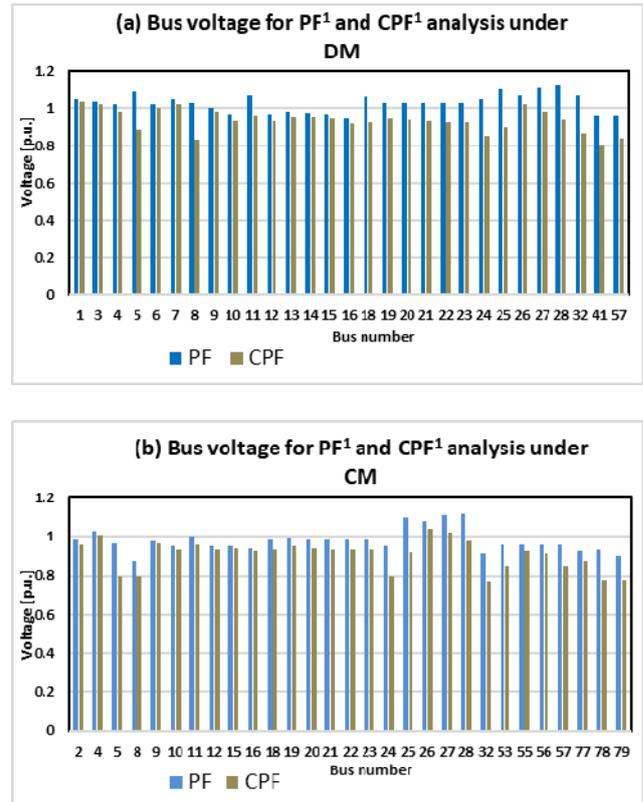
Fig. 9. Power Flow (PF) and Continuation Power Flow (CPF) analysis of the bus voltages
