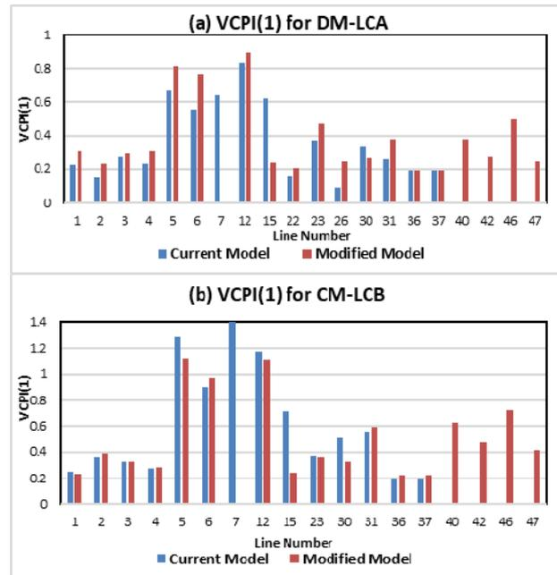
Fig. 14. VCPI comparison between current and modified SIG
