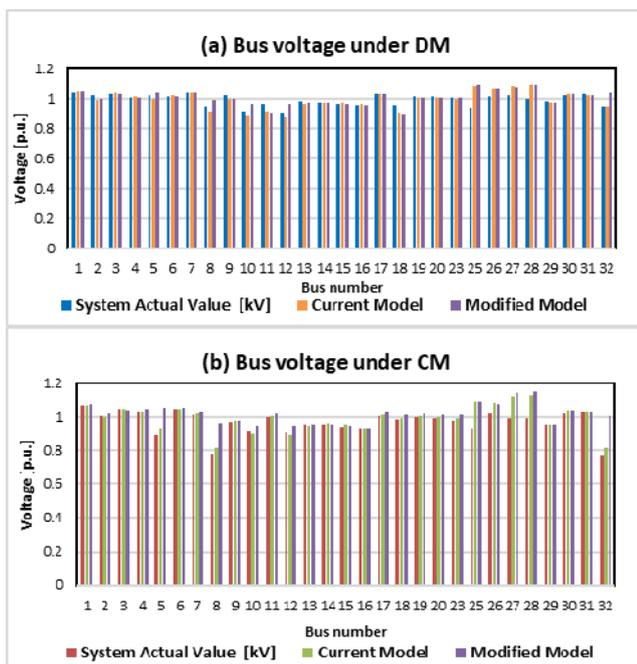
Fig. 18. Bus voltage comparison between actual, current and modified SIG
