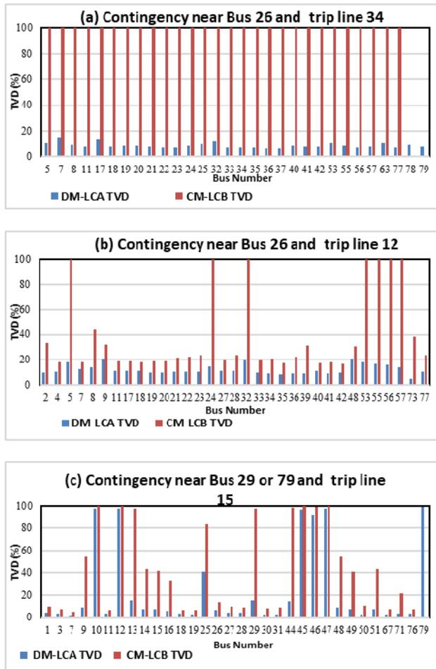
Fig. 10. TVD of the SIG system for contingency near Bus 26 and Bus 29
