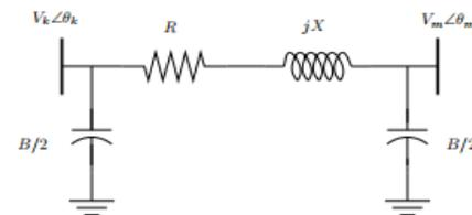
Fig. 7. Transmission line  $\pi$  circuit [18]
