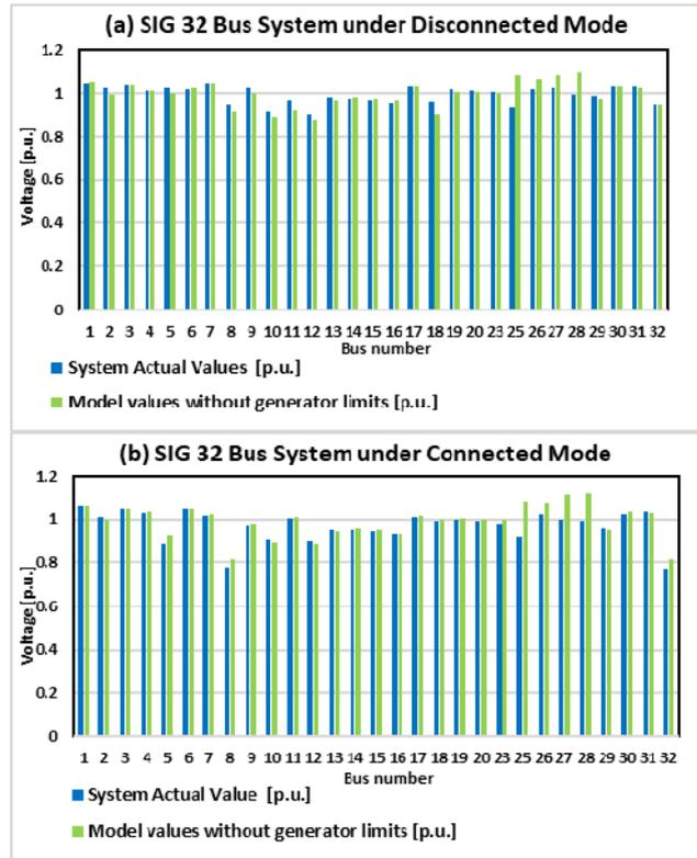
Fig. 8. Comparative analysis between actual and simulated bus voltages
