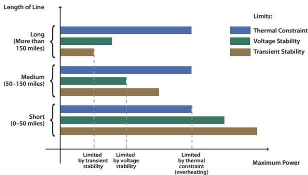
Fig. 1 Three Primary Constraints of Transmission Lines *Invalid source specified..*
