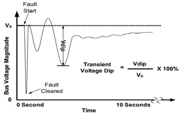
When the transient voltage dip is small and within the voltage stability criteria (25%), the case is marked as healthy or voltage stable. When the largest transient voltage dip is over the voltage stability criteria (25%), the case is marked as voltage unstable [15].
