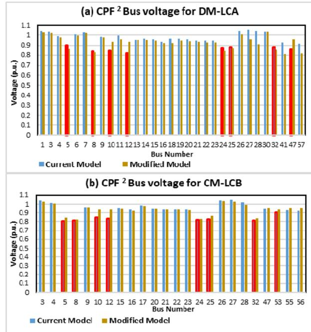
Fig. 13. CPF<sup>2</sup> bus voltage comparison between current and modified SIG
