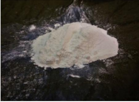
Fig.3 ZnO Nanoparticles sample
