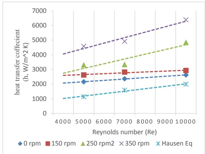
Fig.8 Variation of coefficient of heat transfer with Reynolds number for 0.2% concentration ZnO/water nanofluid using twister tape as working medium
