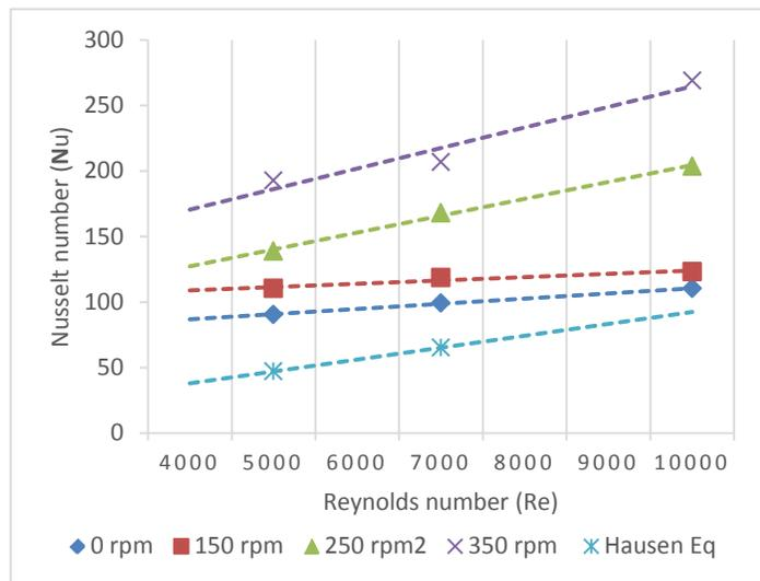
Fig.9 Variation of Nusselt number with Reynolds number for 0.2% concentration ZnO/water nanofluid using twister tape as working medium.
