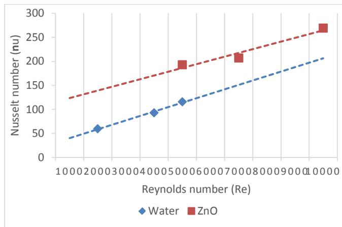
Fig.11 Variation of Nusselt no with Reynolds number for water and ZnO at 350 RPM
