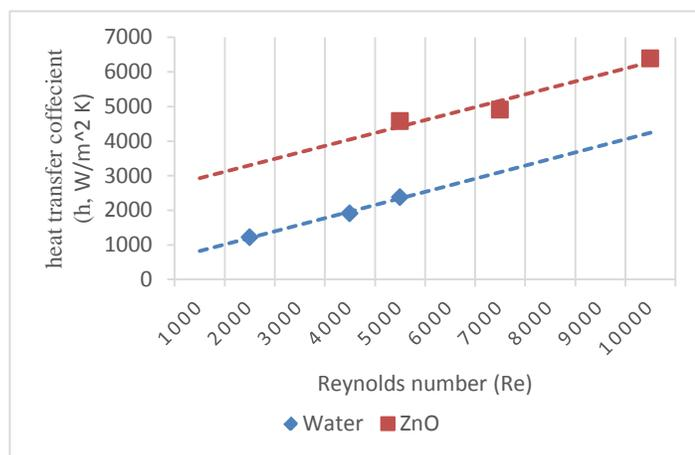
Fig.10 Variation of coefficient of heat transfer with Reynolds number for water and ZnO at 350 RPM
