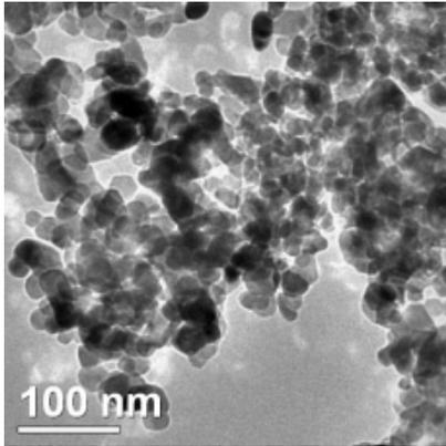
Fig.4 TEM analysis of ZnO nanoparticles
