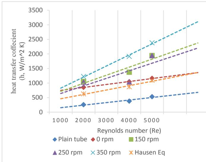
Fig.6 Variation of coefficient of heat transfer with Reynolds number for water as working medium.
