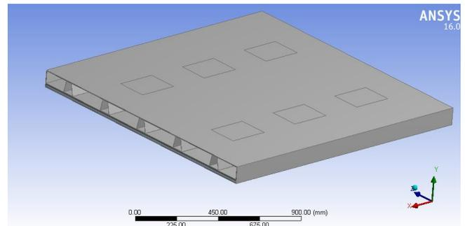
Fig.2 Trapezoidal bridge deck with steel and polyurethane
