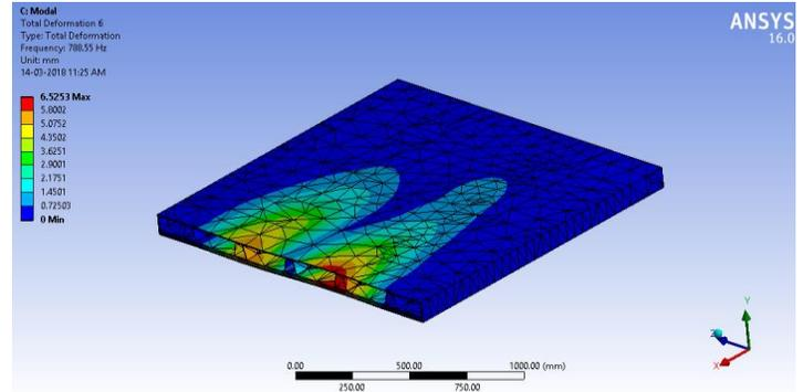
Fig.6 Sixth frequency mode of trapezoidal steel polyurethane bridge deck
