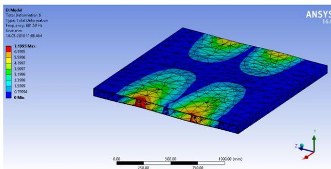
Fig.5 Sixth frequency mode of trapezoidal steel polyurethane bridge deck
