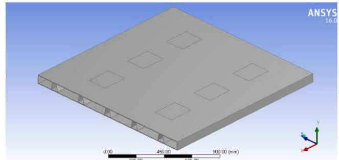
Fig.1 Trapezoidal bridge deck with steel
