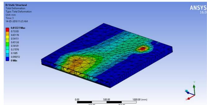
Fig.4 Total deformation in Trapezoidal steel polyurethane bridge deck
