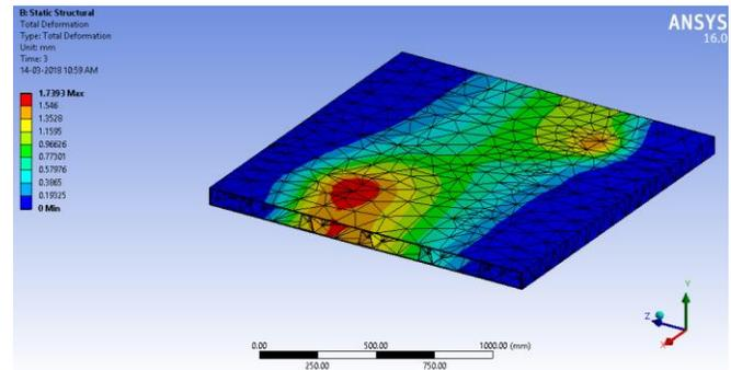
Fig.3 Total deformation in Trapezoidal steel bridge deck
