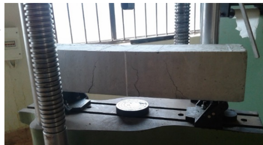
Fig.8. Crack pattern of Normal beam
