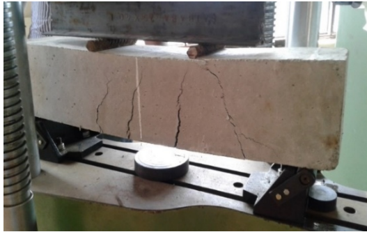
Fig. 9. Crack pattern of ST1
