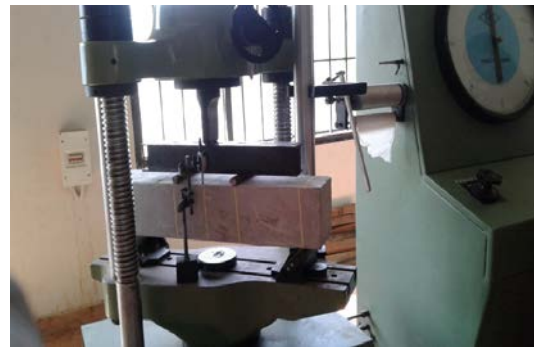
Fig. 5. Flexural Strength Test Setup
