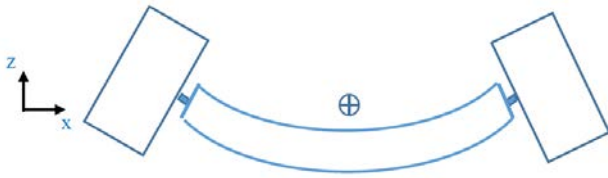
Figure 15. When moving to the left, the lateral tractive forces will bend the chassis and lift the wheels.
