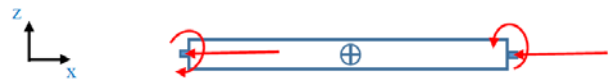
Figure 13. The FBD of the chassis when moving to the left showing forces and moment from wheels to the chassis.
