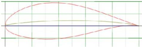
Figure 2. NACA 63415 Airfoil
