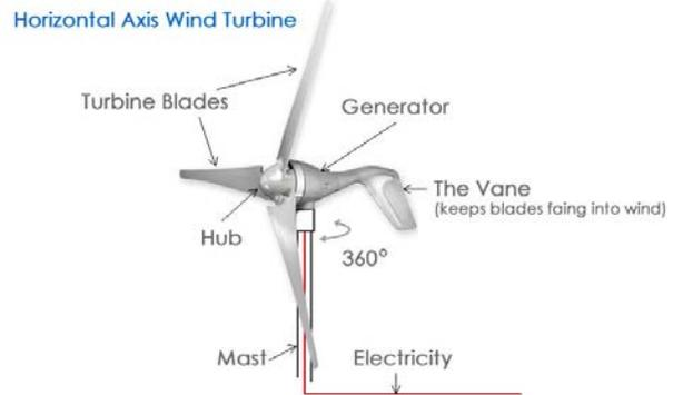
Figure 1 Small horizontal axis wind turbine
