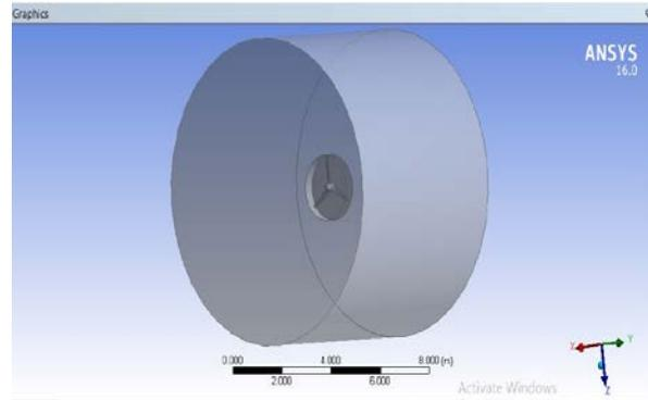
Figure 5. Blade with Outer domain
