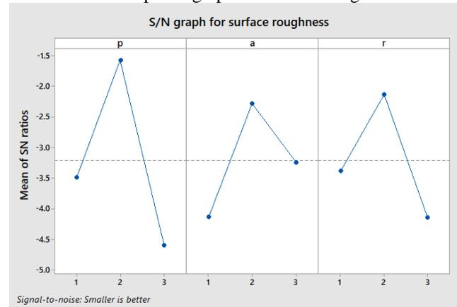
Fig 3. S/N graph for surface roughness
