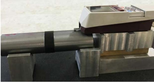
Fig 2. Measurement of surface roughness
