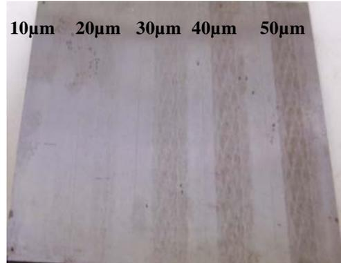
Fig.7 Surface burning from 10µm to 50 µm depth of cut each slot. Table speed 0.12m/s. coolant supply 0.08L/s using NCD.
