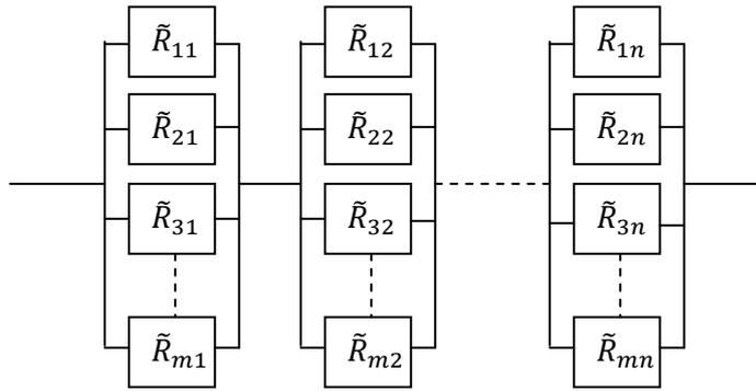
Fig.6 Series-parallel system
