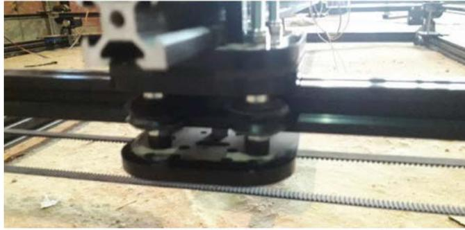
Figure18. Guide wheel holder of y axis
