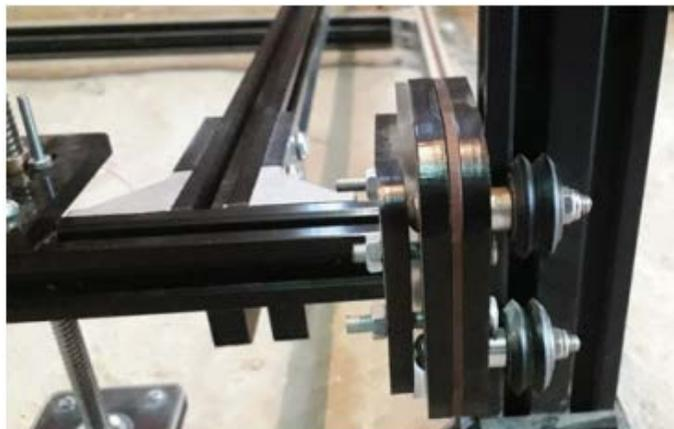
Figure17. Guide wheel holder of Z axis
