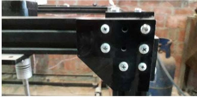
Figure15. Assembly of the corner with assembling part
