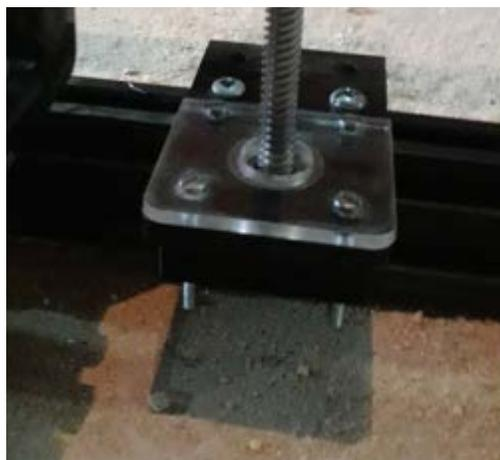
Figure20. Assembly of bearing holders
