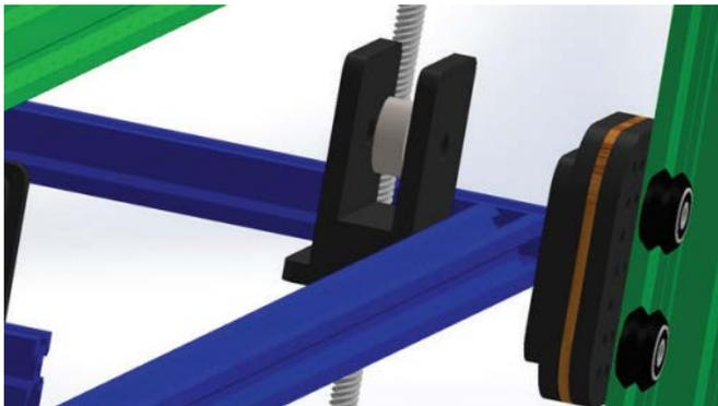
Figure25. Assembly of bearing holders
