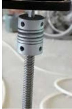
Figure21. Assembly of screw with the coupler with the motor
