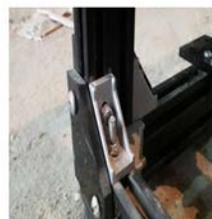
Figure2. b. L-angles for assembly
