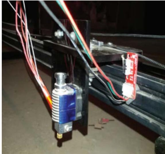
Figure28. Assembly of hot end and laser head
