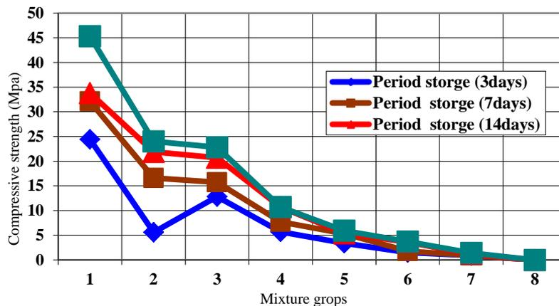
Figure (6) show progress of compressive strength for every grop at period storage for all mixtures with additional light weight aggregate
