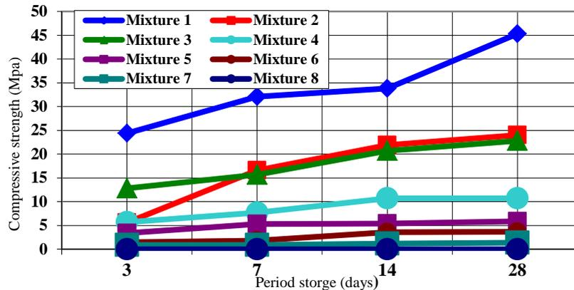
Fig. (5) show relationship between the period of storage and compressive strength for all mixtures with additional light weight aggregate
