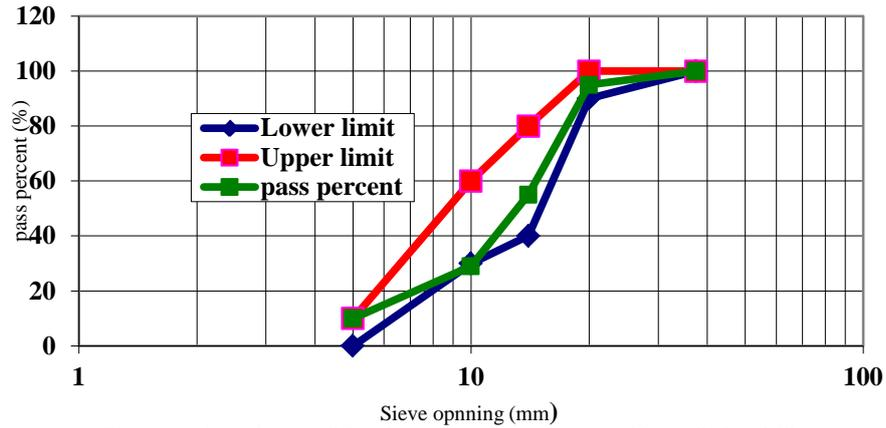
Figure (1) show sieve anylisis of coarse aggregate, upper and lower limits of libyan specification.
