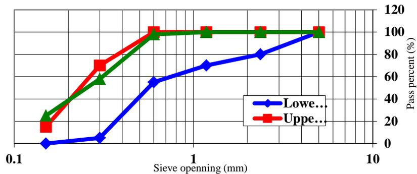
Fig. (2) show the sieve anylisis of fine aggregate and Upper and lower limits of Libyan specifications.
