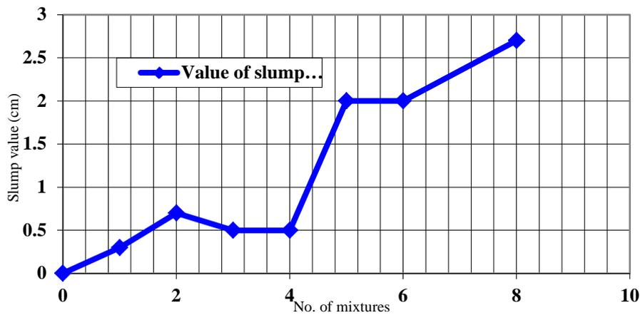
Fig. (3) show the slump of concrete mixtur at added of light wieght ggregate
