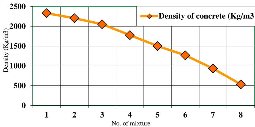
Figure (4) show the density of all mixture with additional light weight aggregate
