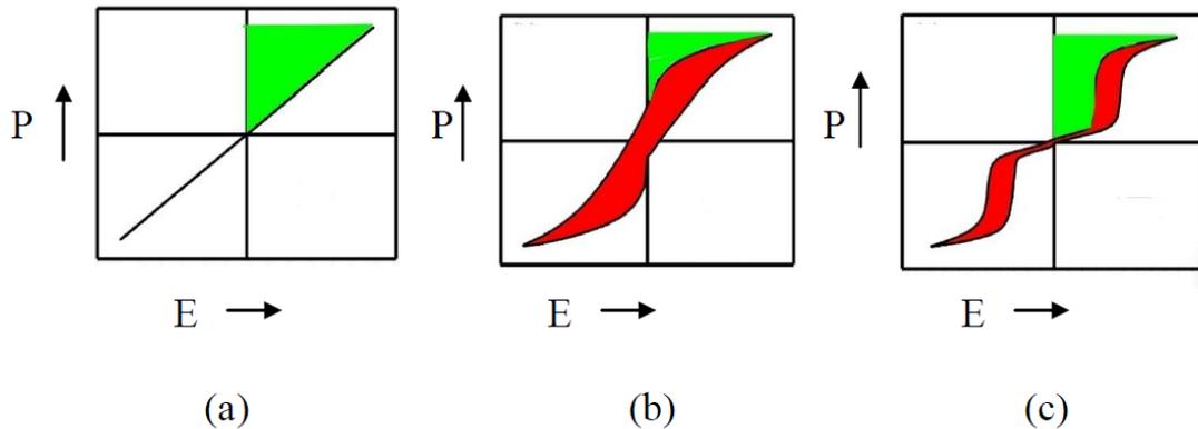
Fig 2. Diagram of hysteresis and energy storage density for (a) linear dielectrics (b) ferroelectrics (c) antiferroelectrics. The green area in the first quadrant is the recoverable energy density  $J_{\text{reco}}$  and the red area is the energy loss  $J_{\text{loss}}$ .
