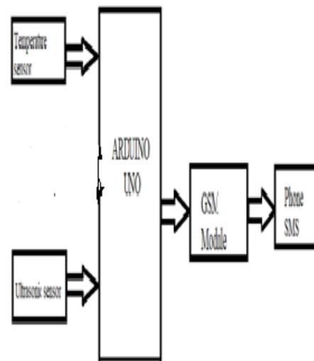
Fig.1 Block diagram
