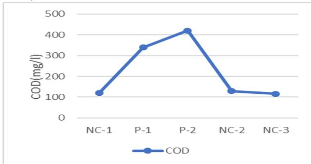
Interferences: The above graph represents the variation of COD (mg/l) of five surface coating industries. COD (mg/l) of phosphating process more than that of nano coating process. The COD value of phosphating process is more than the limit given by CPCB, so the wastewater has to be treated before disposal or reuse.
