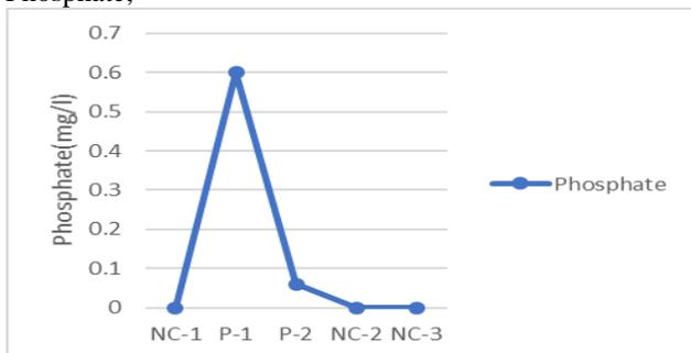
Interferences: The above graph represents the variation of Phosphate (mg/l) of five surface coating industries. Phosphate (mg/l) in nano coating process is nil. The Phosphate value of phosphating process is within the limit given by EPA 2002.
