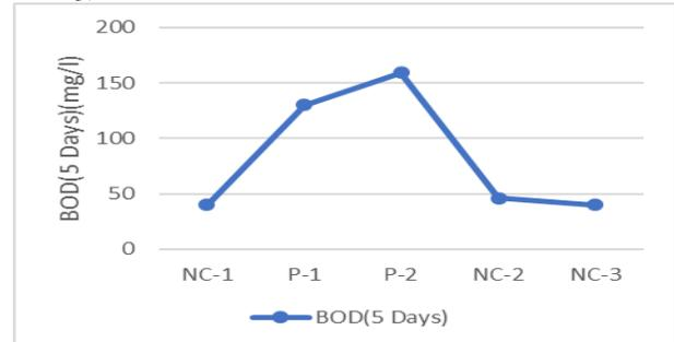
Interferences: The above graph represents the variation of BOD<sub>5</sub> at 20 °C (mg/l) of five surface coating industries.
