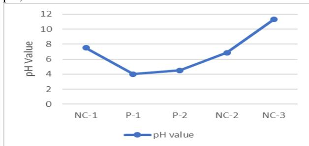
Interferences: The above graph represents the variation of pH values of five surface coating industries. The pH value of phosphating process is acidic in nature and nano coating process is alkaline in nature. The pH value of phosphating process is not within the limit as per CPCB so the wastewater should be treated before disposal or reuse and
