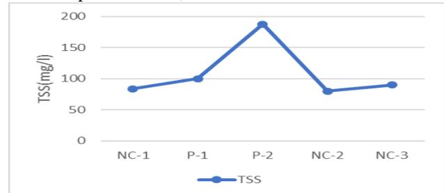
Interferences: The above graph represents the variation of TSS (mg/l) of five surface coating industries. TSS (mg/l) of phosphating process more than that of nano coating process. The TSS (mg/l) of both the processes is more than the limit given by EPA 2002 so both the wastewater should be treated before disposal or reuse.
