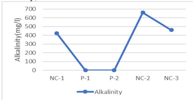
Interferences: The above graph represents the variation of Alkalinity (mg/l) of five surface coating industries. Alkalinity (mg/l) in phosphating process is nil.
