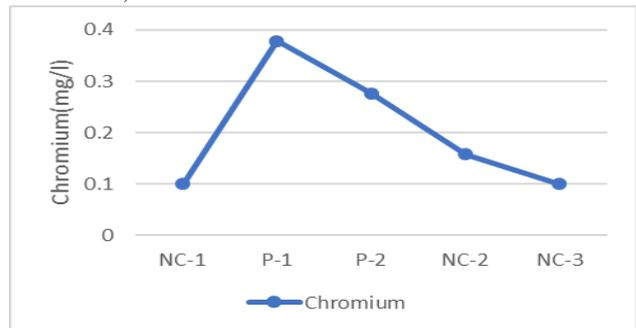
Interferences: The above graph represents the variation of Chromium (mg/l) of five surface coating industries. Chromium (mg/l) in phosphating process is more when compared to nano coating process. The Chromium value of phosphating process is more than the given limit as per EPA 2002 and of nano coating process it is within the limit.
