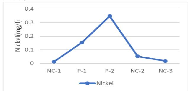
Interferences: The above graph represents the variation of Nickel (mg/l) of five surface coating industries. Nickel (mg/l) in phosphating process is more when compared to nano coating process. The nickel value of phosphating process is more than the given limit as per EPA 2002 and of nano coating process it is within the limit.
