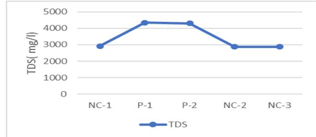
Interferences: The above graph represents the variation of TDS (mg/l) of five surface coating industries. TDS (mg/l) of phosphating process more than that of nano-coating process. The TDS (mg/l) of both the processes is more than the limit given by CPCB so both the wastewater should be treated before disposal or reuse.
