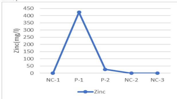
Interferences: The above graph represents the variation of Zinc (mg/l) of five surface coating industries. Zinc (mg/l) in nano-coating process is nil. The Zinc value for phosphating process is more than the limit given by EPA 2002, so the wastewater should be treated before disposal or reuse.
