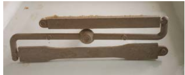
Fig. 2: Injection molded tensile and flexural strength specimen
