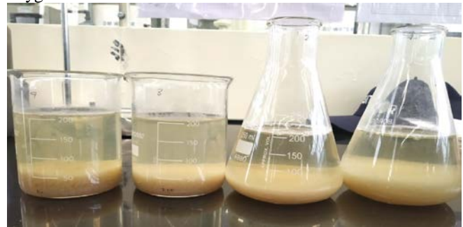
Fig. 2. Settling in process after addition of chemicals.
